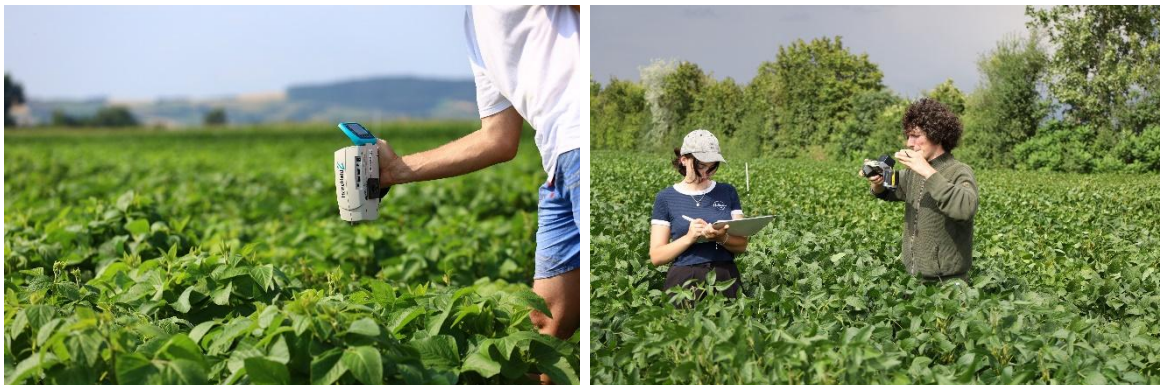
Figure 21. Hyperspectral reflectance (left) and thermographic imaging (right) of Yield-2 plots during early seed filling using hand-held devices for data collection (Photos: BOKU University)
