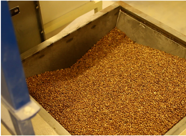
Figure 2. Cleaned and size sorted faba beans fed into silo. Photograph: Casimir Schauman
